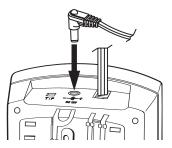
Route the modular cord through either groove on the bottom of the base and the adapter cord through the groove below the strain relief slot.
